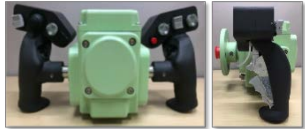
Figure 8: MET-D Crew-station Hand Controller (Yoke) Design Based on User Jury Input
